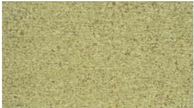
Failed Casing Joint Microstructure After Normalizing at 1,508° (x100)
