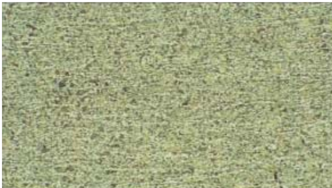
Failed Casing Joint Microstructure After Normalizing at 1,472° (x100)
