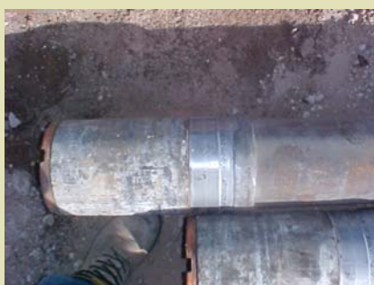
Fig. 3. Wear band crimped on the casing immediately below the casing coupling to protect the coupling from abrasion.
