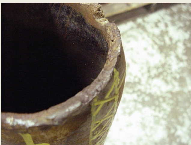
Fig. 3. 45° fracture surface of joint C2.
