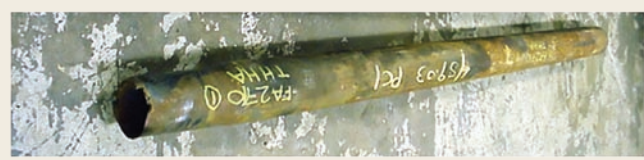
Uphole portion of failed joint
