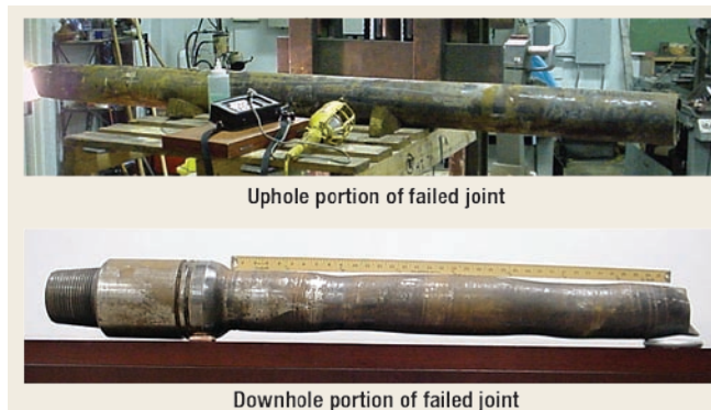
Fig. 1. As received condition of the failed 5-in. 19.50-lb G-105 drill pipe C1.
